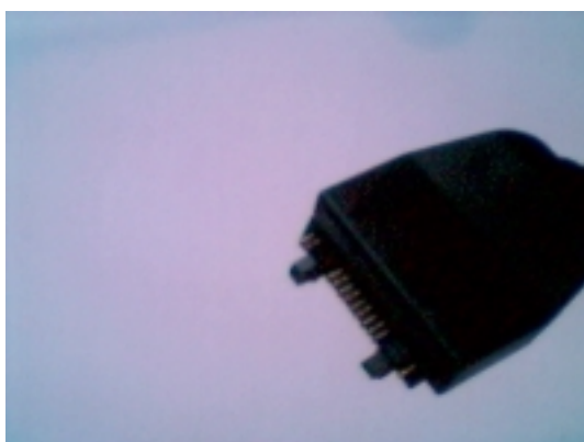
Pic. 1 Connection plug for use with Ericsson A1018#s or T10#s cellular telephones.
