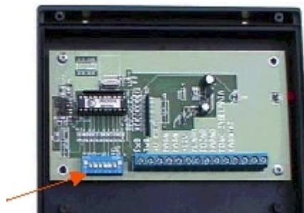
Pic1. Electronic board with microswitch and terminal slot
